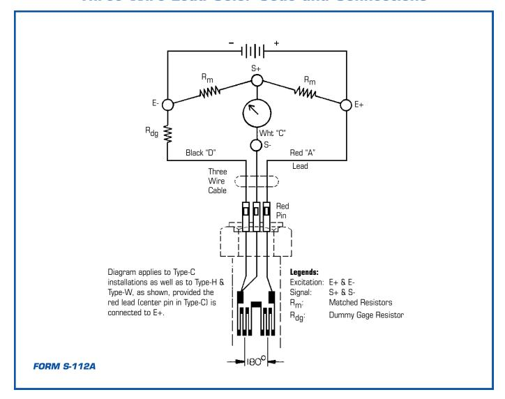
Note: Increasing tension strain in gages induces an increasing signal of positive polarity.
