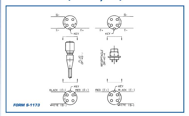
Miniature Connectors do not have pin (A, B, C, D) legends. Various bridge connectors and cable color codes are referenced from Connector Key Position, as indicated herein.
